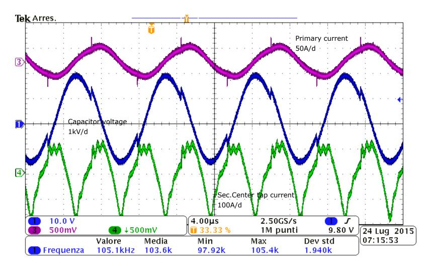
Very close to resonance (~110kHz), waveforms are almost sinusoidal.
