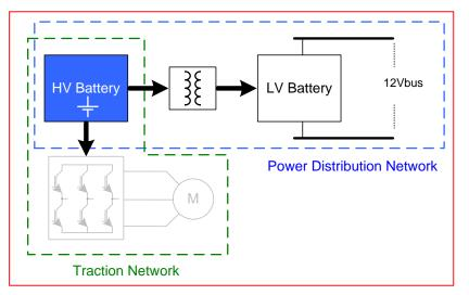
While the traction inverter is directly supplied by the HV battery, all services in a car today still run out of a 12V battery, therefore a HV-DC/DC converter is needed to supply this battery line
