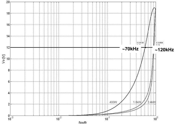
Simulation at Vin = 350V, Vout = 12V and different power output
