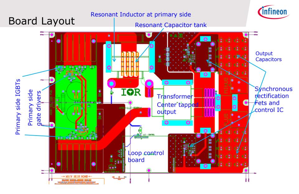
Layout is optmised for system testing and debugging.
