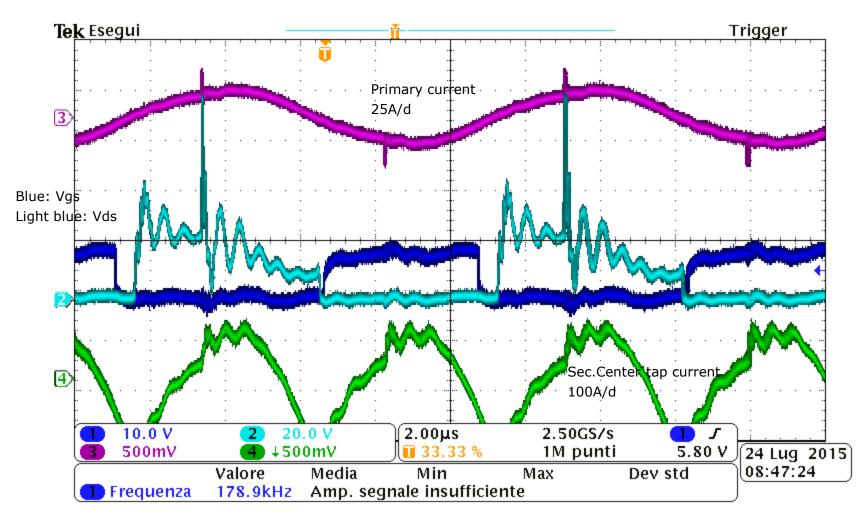
Waveform obtained at high current output of 160A: the signal across the 0,8m  $\Omega$  SR Fets is much more evident as well as switching noise but the gate command signal is regular.
