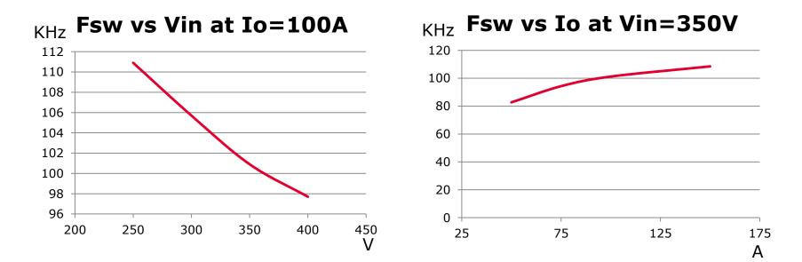
Low switching frequency variation vs. input voltage and load changes Good matching with simulation
