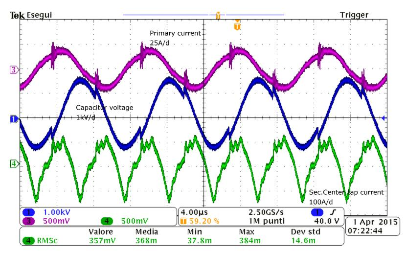
Frequency, capacitors voltage and Primary/Secondary currents increase
