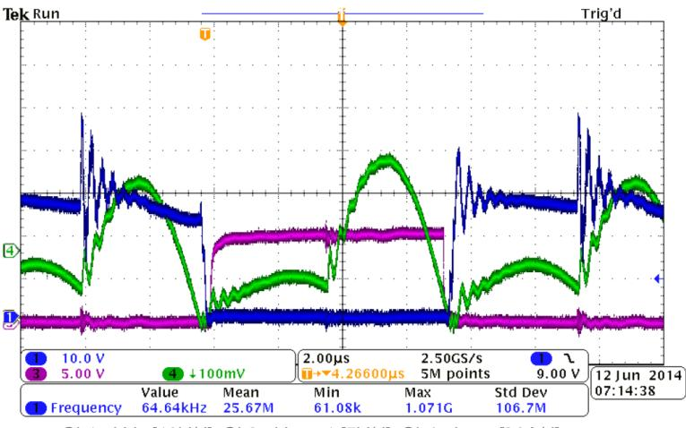
Ch1= Vds [10V/d], Ch3= Vgate1 [5V/d], Ch4= Isec. [20A/d]
