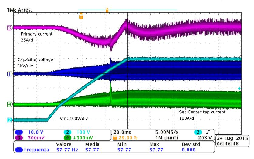
Fast start: Vin rise time is only limited by the Lab power supply Vin=400V, Io=25A
