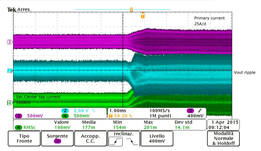
Load increase to 140A (traces 2 and 3 with AC coupling)
