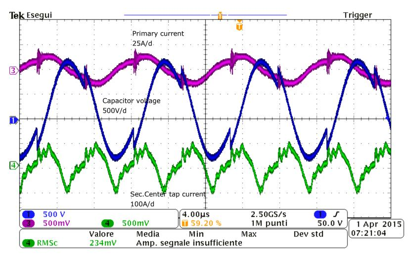
Clean sinusoidal voltage across resonance capacitors, some ringing noise visible on transformer's secondary current
