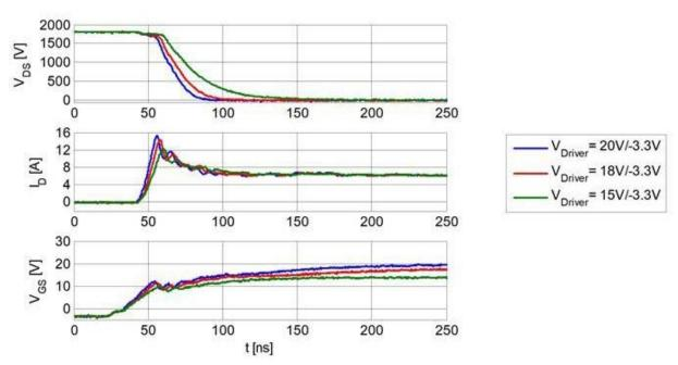
• VDS fall time = 30 ns achieved for switching at 1800 V and 6 A, with +20 V drive voltage and RG,ext = 10  $\Omega$
