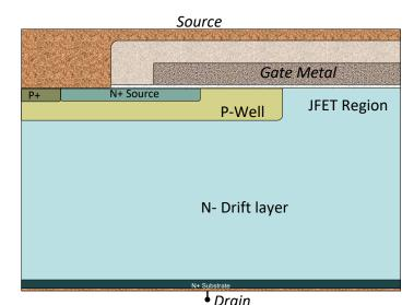
Standard DMOSFETs for highly uniform production and robust and reliable performance
