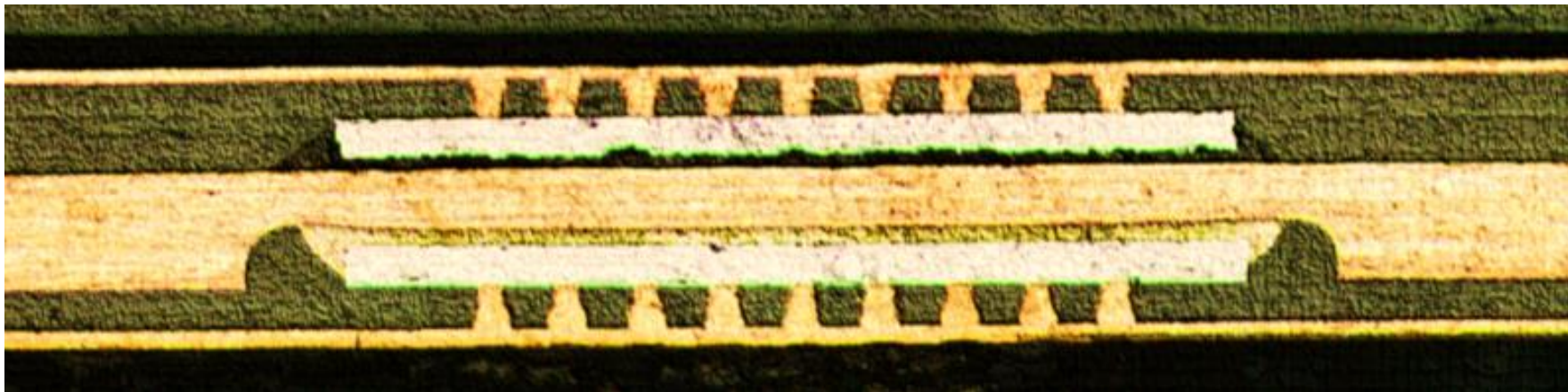
P 3 – Stack (3D stacking in Chip Embedded Structure)
