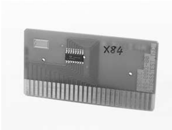
Figure 11. SOIC Unit From Subcon A Soldered to PWB
