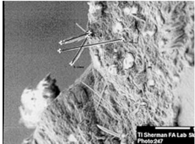
Figure 24. Subcon A SOIC Unit at 1400X, 3000-Hours Exposure to Run-4 Conditions (No Precondition, Bias + 51°C/85% RH). Inspection Location 4. Multiple Whiskers Noted, With Length = 8.0–17.7 μm.
