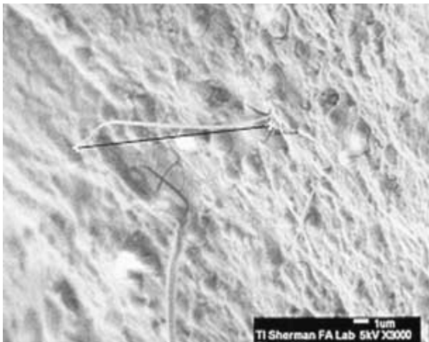
Figure 19. Subcon A SOIC Unit at 3000X, 2000-Hours Exposure to Run-4 Conditions (No Precondition, Bias + 51°C/85% RH). Inspection Location 4. Whisker Length = 12.4 µm.
