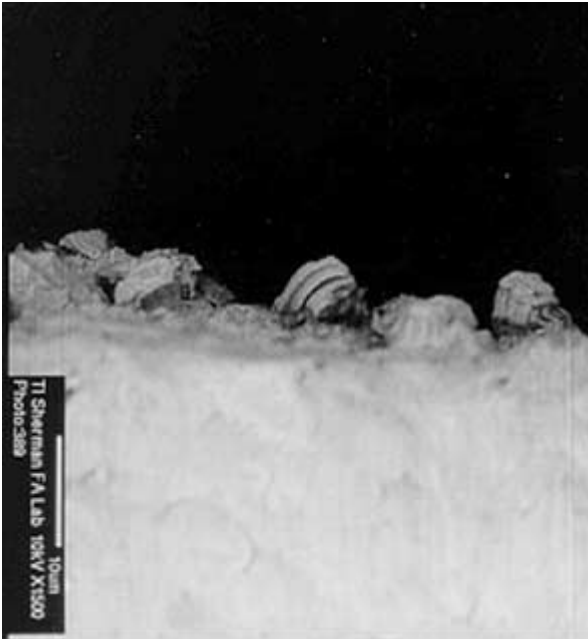
Figure 45. Subcon F SnBi-Finished SOT Package After 3634-Hours Exposure to 51°C/85% RH. Inspection Location Left Edge, Foot Area. Multiple Whiskers Noted, Length = 5.7–6.5 \mu\text{m} .
