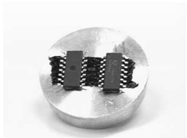
Figure 12. SOIC Units Glued to SEM Inspection Pedestal Prior to Test-Condition Exposure
