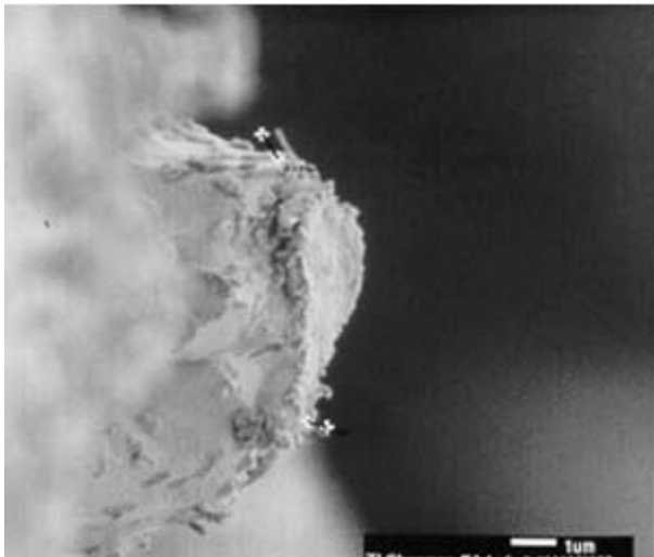
Figure 43. Subcon F SnBi-Finished SOT Package After 3634-Hours Exposure to 51°C/85% RH. Inspection Location 1, Right Side. Whisker Length = 0.4–0.6 μm.
