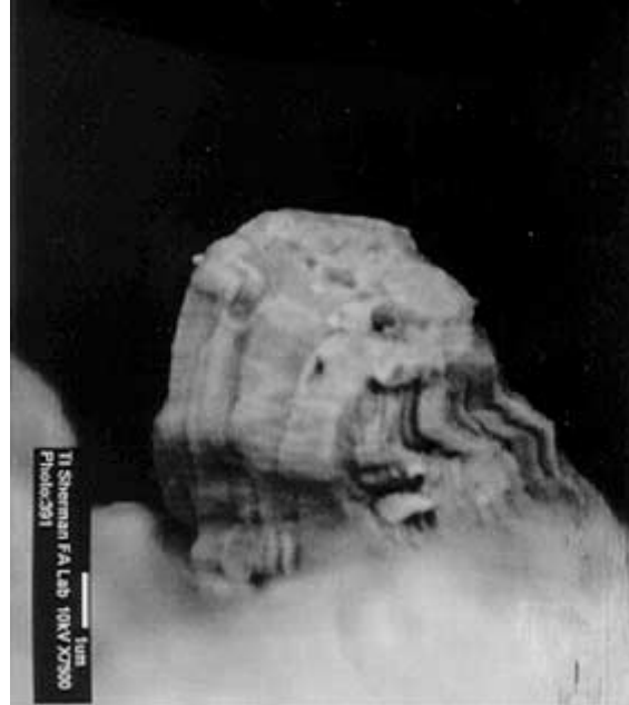
Figure 46. Subcon F SnBi-Finished SOT Package After 3634-Hours Exposure to 51°C/85% RH. Inspection Location Left Edge, Foot Area. Closeup of Whisker, Length = 6.5 \mu\text{m} .
