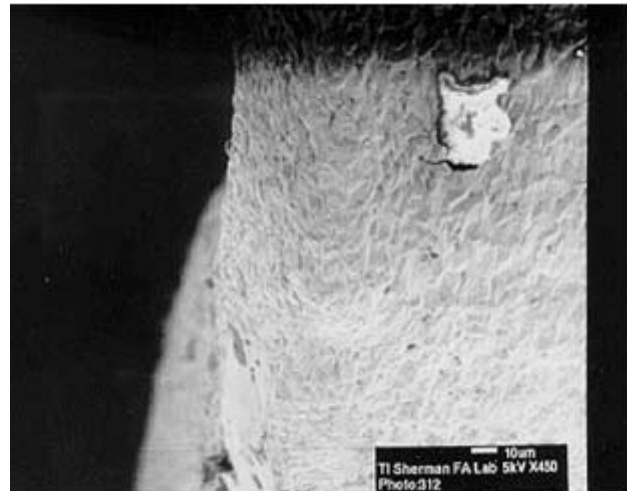
Figure 40. Subcon D SOT Unit at 450X, 3634-Hours Exposure to 51°C/85% RH, Unbiased. Inspection Location 1. No Whiskers Noted.
