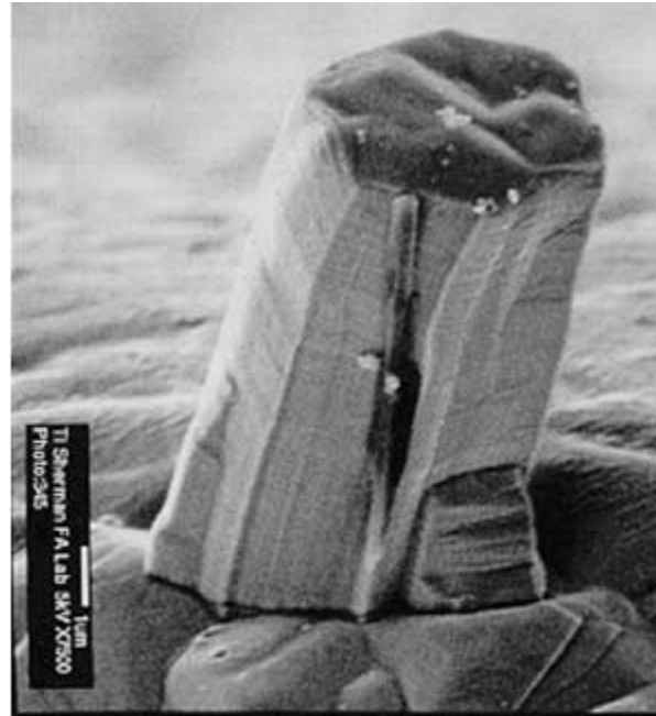
Figure 30. Subcon C TO-220 Unit at 7500X, 3634-Hours Exposure to Precondition + 51°C/85% RH, Unbiased. Inspection Location 7, Right Side. Whisker Length = 9.3 μm.
