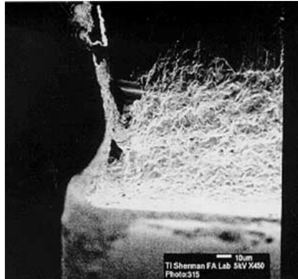
Figure 28. Subcon B SOT Unit at 450X, 3634-Hours Exposure to 51°C/85% RH, No Precondition, Unbiased. Inspection Location 1, Right Side. No Whiskers Noted.
