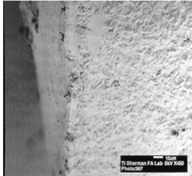
Figure 18. Subcon A SOIC Unit at 450X, 1000-Hours Exposure to Run-4 Conditions (No Precondition, Bias + 51°C/85% RH). Inspection Location 1. No Whiskers Noted.
