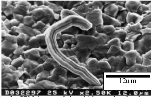
Fig. 2 SEM image of tin whisker under the thermal shock stress
