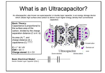
Ultracapacitors are also known as supercapacitors or double layer capacitors
