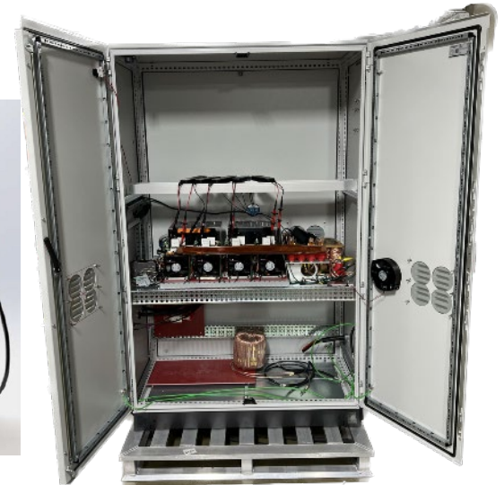
1kV 500+ kW charger
