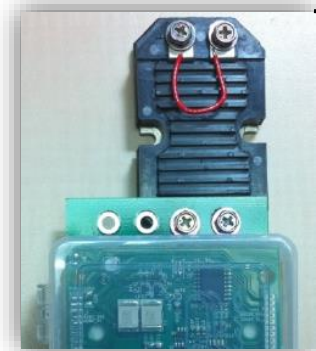
13kV SiC MOSFET based SST with Inductor (4mH) integrated coaxial winding transformer
