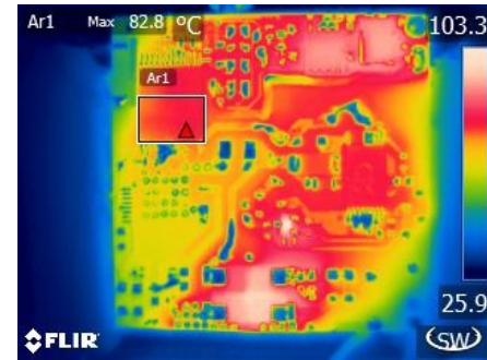
Primary main switch temperature = 82.8 °C
