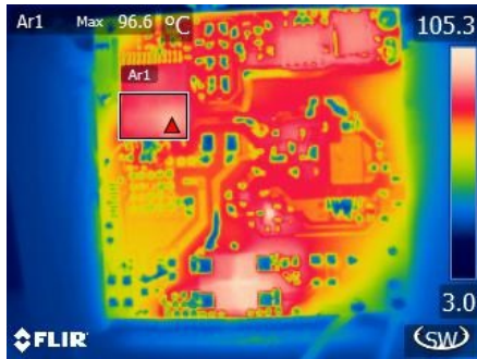
Primary main switch temperature = 96.6 °C
