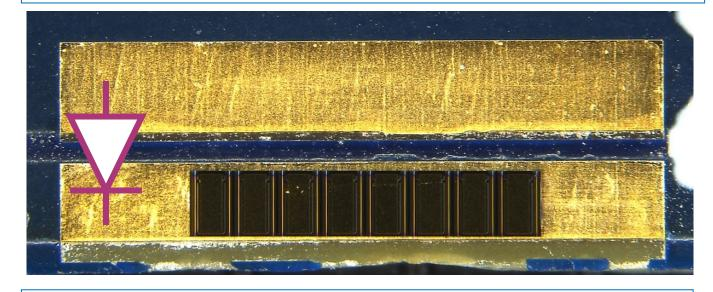
Step 2: Mount copper clip to laser bar anodes & to PCB with conductive epoxy
