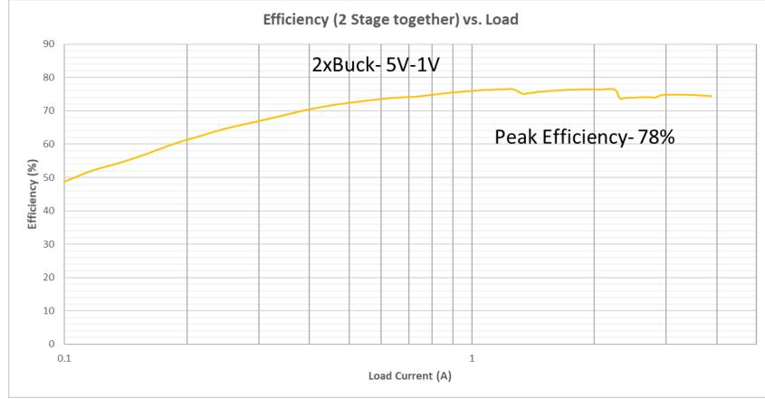
• Peak efficiency of 78% when pre-regulator and IVR are together
