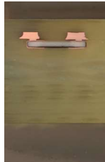
Microsection of gate resistor on L2
