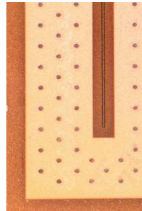
Surface polishing down to microvia contacts
