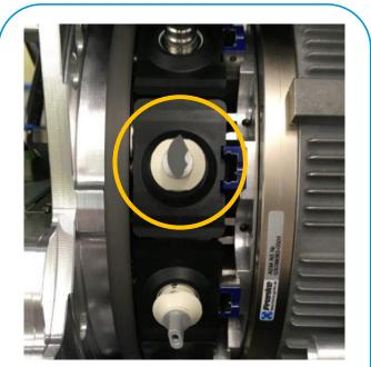
Pick up nozzle with inlay part on assembly head
