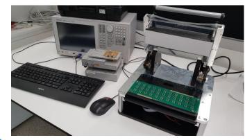
Semi-automated measurement includes test fixture and impedance analyser to gain results.
