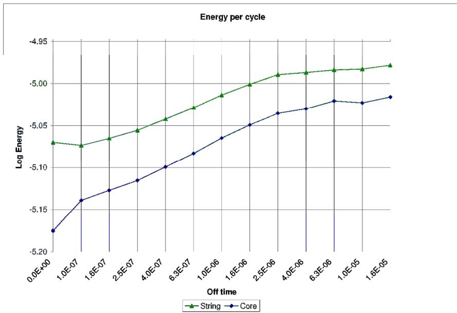
This graph shows the same data, except the energy per cycle is shown logarithmically. On the log-log graph, the slope of the curve for the “string of beads” can be seen to be lower, particularly for small off times. With so little data, it is impossible to assess the significance of this. It may or may not be repeatable, but it suggests a lower proportionate increase in core loss per cycle with added off time for the “string of beads” configuration.
