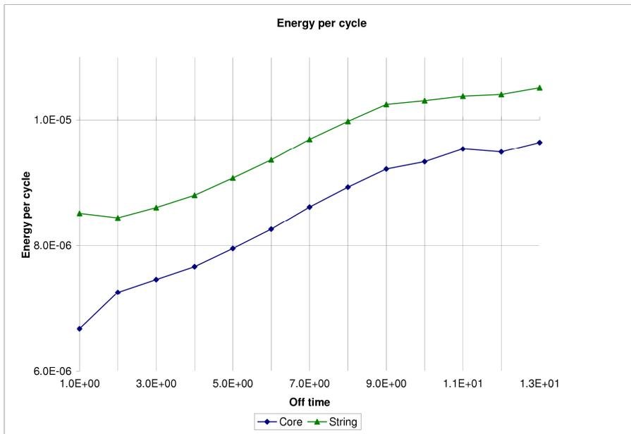
These data and graph show the energy per cycle for the core, in blue, and for the string of beads, in green. The pulse width is a constant 3.98  $\mu$ s. Except for the first data point, the curves are quite similar.
