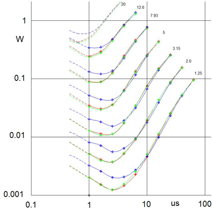
If a string of beads were made with more cores, the flux density would be lower in each, suggesting that the losses would be lower as well. On the speculation that the curves would have the same shape but lower core loss, they would be vertically displaced by the proportionate power difference, as it is a log-log curve.
