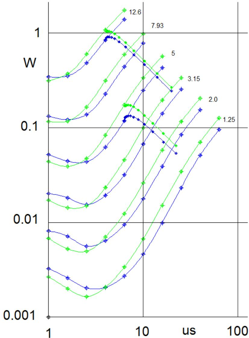
The blue curves are the baseline core, using the data from the mi12-2 run set.. The green curves are the 42 string of beads, using data from the mi12-3 run set.
