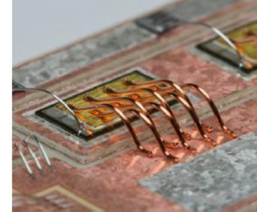
Wolfspeed MOSFET with sintered top plate
