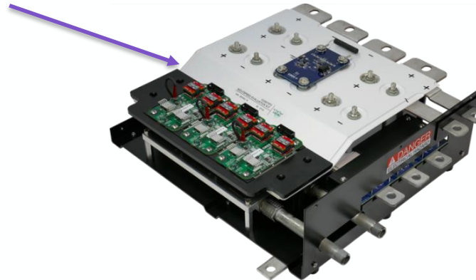
Design with optimized DC laminated Bus structure
