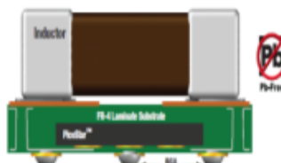
MicroSiP™ cross-sectional view
