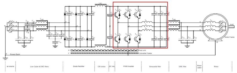
Example of resonant switching cells used in drive for EMC sensitive environments.
