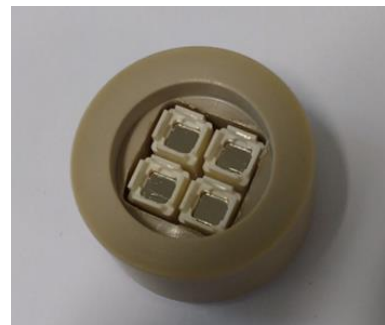
Fig. 7: Prototype of a multichip press-pack SiC Schottky diode
