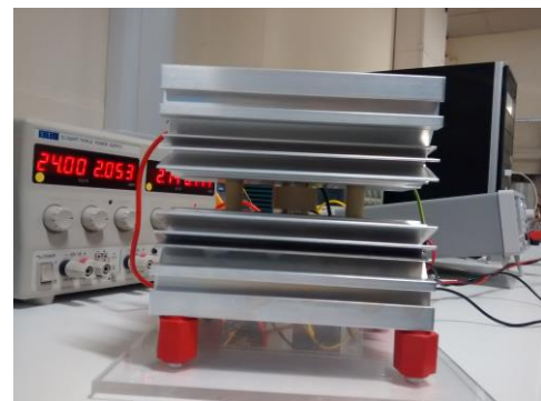
Fig. 8: Double side heatsink assembly for DC heating tests
