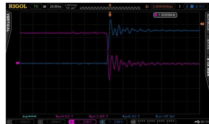
Turn-off (on) characteristics of lower (upper) HEMT
