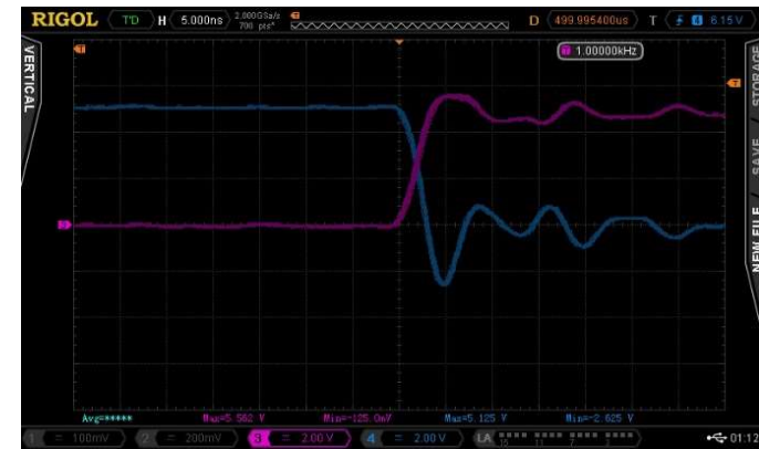
Turn-on (off) characteristics of upper (lower) HEMT
