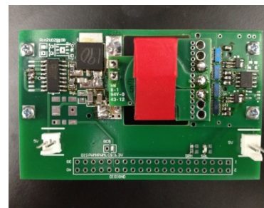
HV IBC: 300 W, 400 V to 12 V GaN devices
