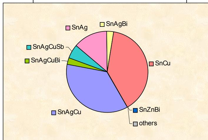
Figure 6: Alloys for hand soldering
