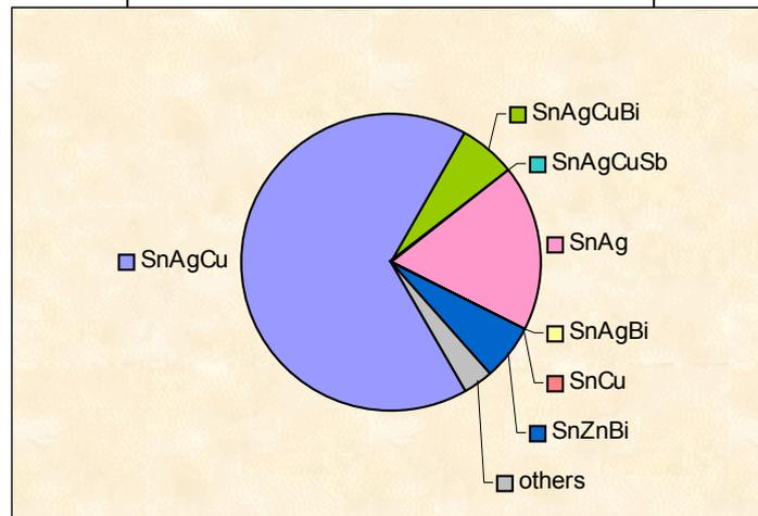
Figure 5: Alloys for wave soldering
