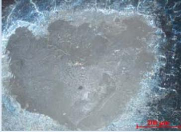
When dielectric breakdown occurs at a fault point, the electrode is vaporized around the point and the capacitor continues to function normally.
