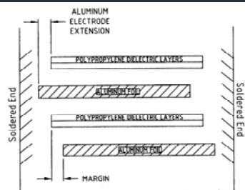
Here is a schematic of a film with metal foil construction. You can see the discrete foils independent from layers of polypropylene film. In this drawing, you can see the aluminum foil ends are soldered to make a connection. It is also common practice to attach to the foil ends with other mechanical connections if the currents are not too high.
