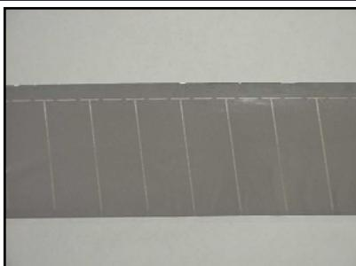
Here is an example of a typical segmented pattern on a metallized film. You can see the film surface is divided into multiple independent areas. You can see that there are little open areas, which can be called gates for current to flow thru. These gates are devices that act like fuses. In their case, when a large fault or self-healing occurs they close and prevent further current from flowing in that region. Thus, the region is isolated with only a smaller amount of capacitance reduction.
