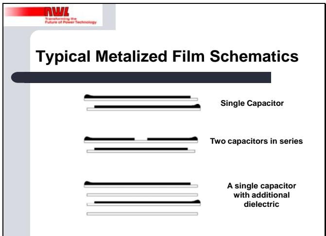
Here are some additional examples of metallized film schematics. You can pattern the metallization in many ways for higher voltage applications. On the top, you can see a single capacitor. You can also have two capacitors in series, which can increase the voltage, or you can increase voltage by adding additional layers of plain film dielectric.
