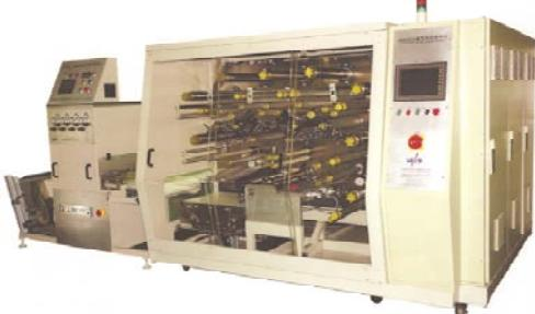
Here is a photo of a piece of winding equipment that is used for making high voltage capacitors with film dielectric and aluminum foil electrodes. This allows a capacitor element to be made in an automatic repeatable fashion including the folded foil attributes for partial discharge elimination.
