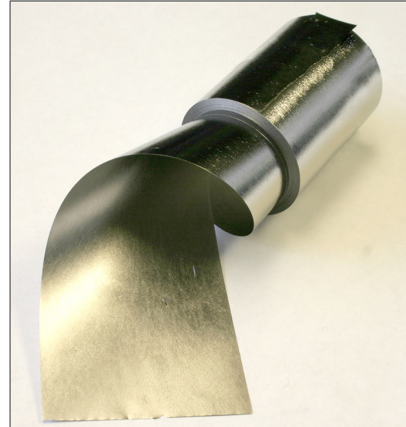
As-Cast Amorphous Metal Ribbon
