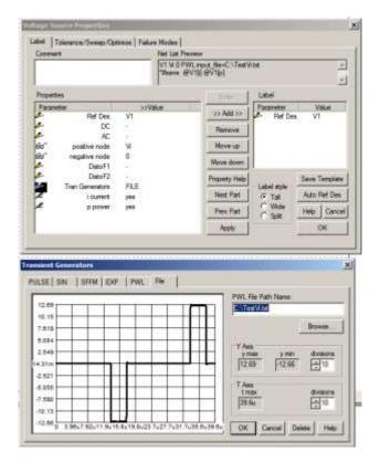
Open the voltage sources, each in turn, select Trans, then File and select the file to which the data has been saved. (Alternatively, open PWL and copy and paste the data.)
