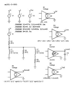
**Note:** The core loss SPICE model is different. This illustration is to show the added functions. The simulation examples that follow use this model, and it is not as good as the simple mode.
