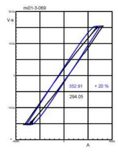
Expanded excittion, with an off-time of 0.125  $\ensuremath{\mu s}.$
