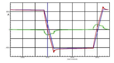
The scale factors of the traces can be set in the SPICE oscilloscope. The Dif function makes the current difference easier to see. In particular, the vertical distance between the sloped lines is very hard to visualize. Dif shows a much greater error there than is apparent to the eye.
