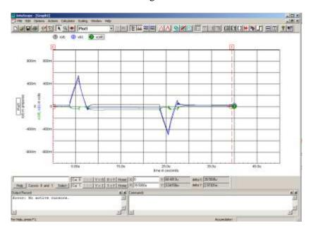
The hysteresis curve for the model vs the data is shown below. The blue hysteresis loop is from the SPICE model and the black hysteresis loop is using the .csv data input current, both with the .csv input flux as the vertical axis. By taking the ratio of the areas inside the hysteresis loops, we find that the model estimates the loss about 12 percent low. The qualitative behavior is quite well matched.
