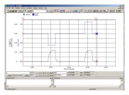
The picture below shows the energy loss, the energy stored and the total energy over the cycle <u>in the SPICE model</u>. The energy loss in the SPICE model should equal the energy calculated from the measured data, and it is quite good. The value from the graph can be seen at the bottom as Cur 1 Y = 9.18u. The calculated energy from the data is 9.16E-6 J. This close match exists because the model is running with the same excitation conditions that were used to make the model.
