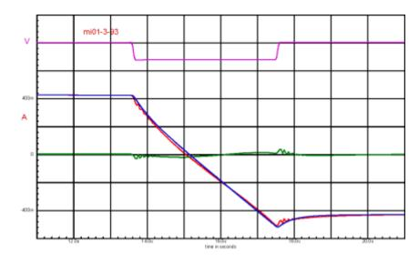
The difference current display is particularly valuable in showing that the error (the difference current) is about the same when excitation is applied as when it is removed. This suggests that the off-time core loss phenomenon is mis-named. It is there during the on time as well. This suggests that transition time core loss is a better name.
