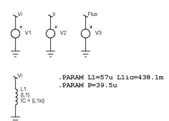
I added a parameter .PARAM  $\{L1ic\} = 438.1 \text{ m}$ . I also added a .PARAM P=39.5u. The parameter  $\{P\}$  is the period, and can be used to set the run time in the Simulation Setup.
