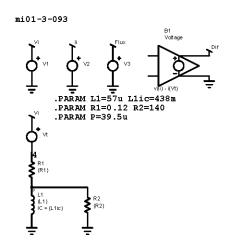
The model is significantly improved. The Dif error is much less than it was. Note that the slight slope error on the left is now gone. The contribution of R1 is small, but is important for simulating longer off-times. The contribution of R2 is greater. The amplitudes of the currents are now quite well matched, but the time constants are mismatched.
