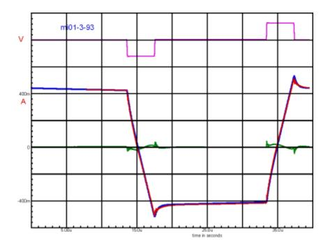
The current match between the data and the simulation is now fairly good. Notice that the error in the Dif current is not zero, but has nearly equal area above and below 0. There will be a slight error in the shape of the hysteresis loop, but the area within it should be quite close.
