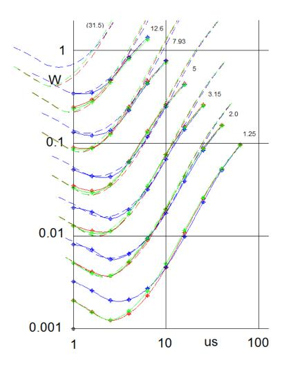
In the graph above, the 1 volt curves were copied, changed to dashed lines, then pasted on the higher voltage curves by eye to make the best fit. The fit is qualitatively fairly good for points for which there are data. Whether this is valid at shorter pulse-widths is highly speculative, but it may show the general shape of the curves.
