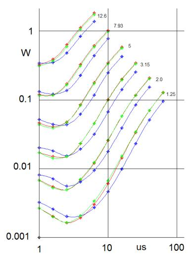
There is not much cross-over at the highest voltage test, but loss difference is more than is apparent because it is difficult to see small differences on a log-log plot of several decades. The 500 kHz test with 12.55 V is as follows:
