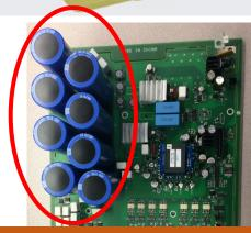
100A VFD – 8 x ? $\phi$  x ?H capacitors
