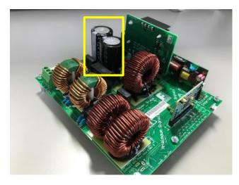
Aluminum Electrolytic Capacitor Is The Relevant Component Of The Overall PSU Life Time!!!!
