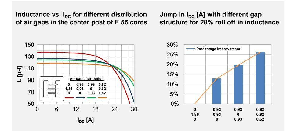
The delayed core saturation is realized due to the lower temperature rise which is around 1/3<sup>rd</sup> for wire coil
