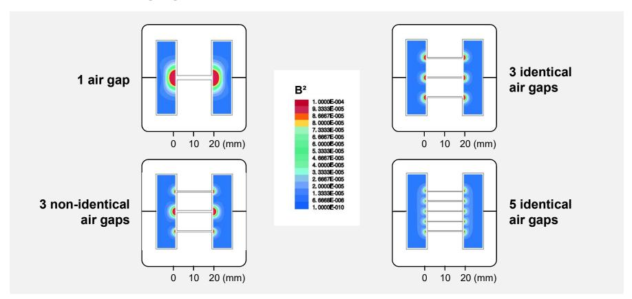
Loss due to fringing flux get decreased in proportion to B<sup>2</sup> with an increasing number of identical air gaps
